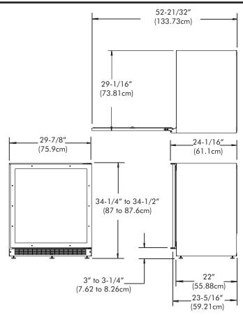
Rough In Opening Dimensions for 8SBARE Glass Overlay Door
