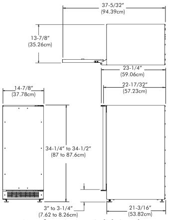
Rough In Opening Dimensions for 3SBARE Solid Overlay Door
