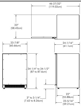
Rough In Opening Dimensions for 6SBARE Solid Overlay Door
