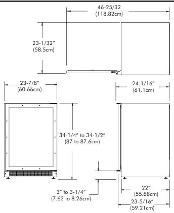
Rough In Opening Dimensions for 6SBARE Glass Overlay Door
