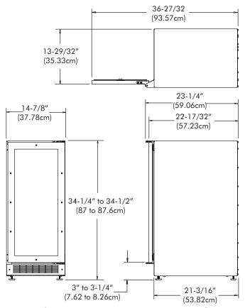
Rough In Opening Dimensions for 3SBARE Glass Overlay Door
