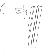
Remove the two outside screws holding door / drawer handle.
