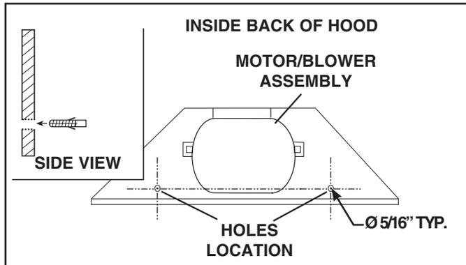
12. With the hood hanging in place, drill through both holes located in the inside lower back of hood using a  $\frac{5}{16}$ " drill bit. Insert the included drywall anchors into the drilled holes (one for each hole). Install (2) washers and (2) #8 x 1-1/2" mounting screws through the hood back and into the drywall anchors. Verify that the hood is centered and leveled. Tighten all screws completely.
