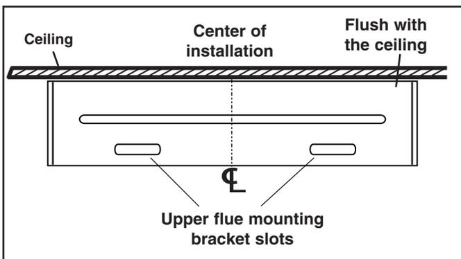
1. Drill two  $\frac{5}{16}$ " diameter holes where shown. Insert drywall anchors into the holes.
