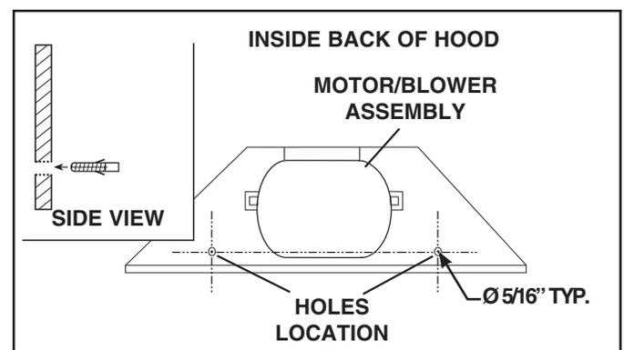
8. With the hood hanging in place, drill through both holes located in the inside lower back of hood using a  $\frac{5}{16}$ " drill bit. Insert the included drywall anchors into the drilled holes (one for each hole). Install (2) washers and (2) #8 x  $1\frac{1}{2}$ " mounting screws through the hood back and into the drywall anchors. Verify that the hood is centered and leveled. Tighten all screws completely.
