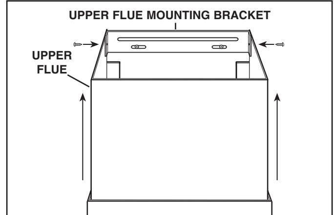
14. Slide the upper flue upward until it is aligned with its upper mounting bracket. The bracket should be inside the flue. Secure the upper flue to the upper flue mounting bracket using (2) #8 x 3/8" mounting screws.
