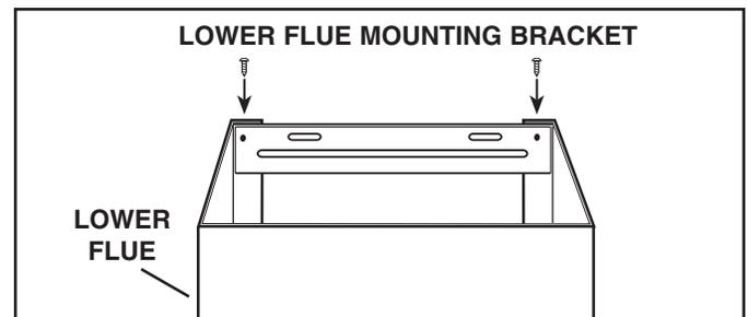
**NOTE: 10-ft. ceilings require 10-ft. Flue Extension Model FXN58SS (purchase separately). Discard the upper flue supplied with your hood and replace it with the Model FXN58SS flue extension.**
