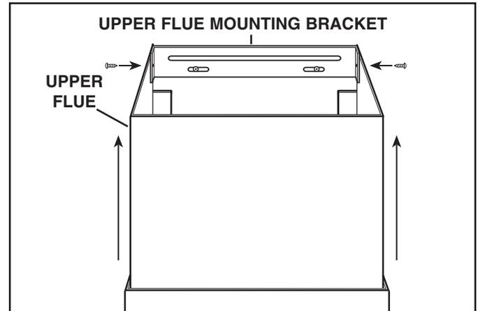
15. Slide the upper flue upward until it is aligned with its mounting bracket. The bracket should be inside the flue. Secure the upper flue to the upper flue mounting bracket using (2) #8 x 3/8" mounting screws.
