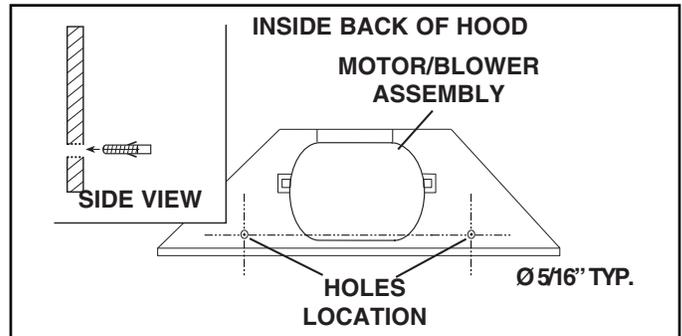
16. With the hood hanging in place, drill through both holes located in the inside lower back of hood using a 5/16" drill bit. Insert the included drywall anchors into the drilled holes (one for each hole). Install (2) washers and (2) #8 x 1-1/2" mounting screws through the back of the hood and into the drywall anchors. Verify that the hood is centered and leveled. Tighten all screws completely.
