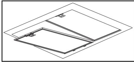
7. Attach non-duct collar to non-duct plenum using (4) ST4 x 8 round head screws.
