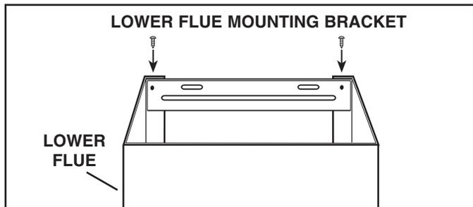
11. Remove the upper flue from inside the lower flue. Install the lower flue bracket to the lower flue using (2) flue bracket screws #8 x 3/8", make sure that the slots are at the top. Carefully replace the upper flue inside the lower flue. Remove protective plastic film covering the lower flue only.
