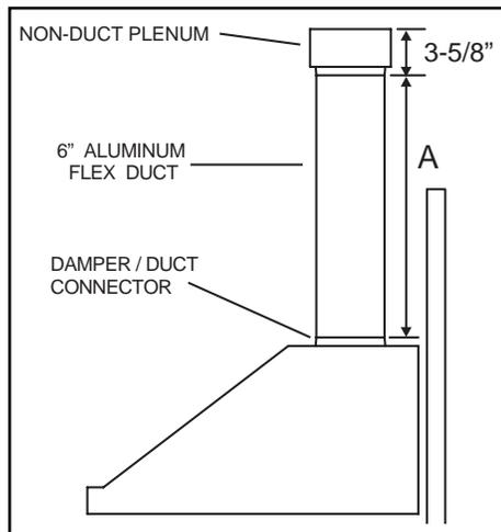
**NOTE: 10-ft. ceilings require 10-ft. Flue Extension Model FXN58SS (purchase separately). Discard the upper flue supplied with your hood and replace it with the Model FXN58SS flue extension.**
