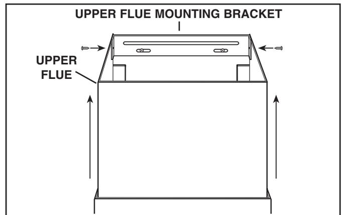
19. Slide up the upper flue upward until it is aligned with its mounting bracket. The bracket should be inside the flue. Secure the upper flue to the upper flue mounting bracket using (2) #8 x 3/8" mounting screws.
