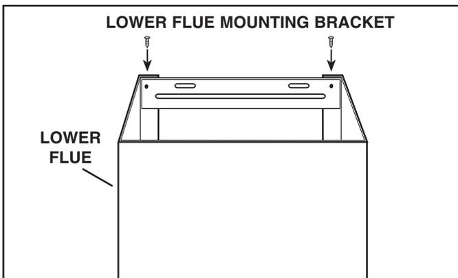
**NOTE: 10-ft. ceilings require 10-ft. Flue Extension Model FXN58SS (purchase separately). Discard the upper flue supplied with your hood and replace it with the Model FXN58SS flue extension.**
