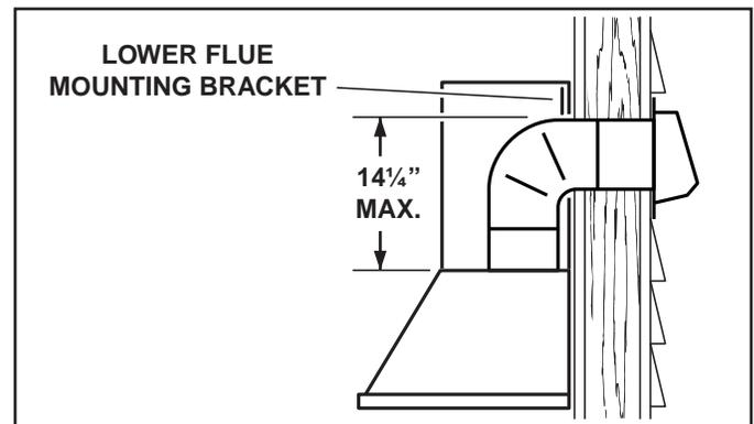
6. To make sure there will be adequate clearance between top of hood and lower flue mounting bracket for ductwork: Elbow must be located below lower flue mounting bracket.
