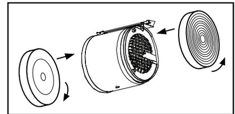
For replacement non-duct recirculation filters - purchase S97018030 or ROUNDFILTER.
