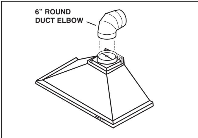
10. Measure and install 6" round steel ductwork to roof cap or wall cap and 90° elbow over duct collar on hood. Use duct tape to make all joints secure and air tight.
