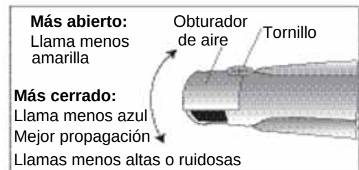
FIGURA 25: AIR SHUTTER ADJUSTMENT (IF NECESSARY)
