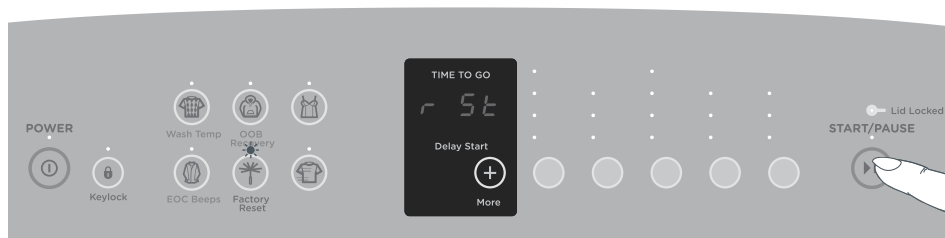
Fig.38 Changing the washer back to the factory default settings
