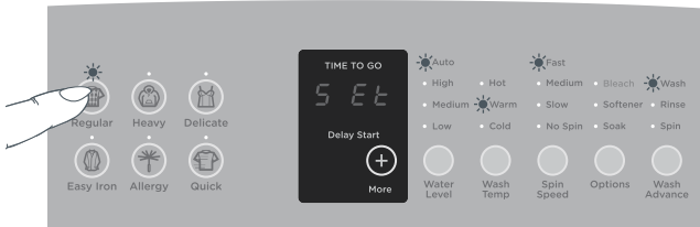
Fig.31 Customizing a wash cycle, eg REGULAR cycle
