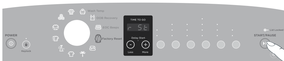
Fig.33 Changing the washer settings back to the factory default (WL4027P)
