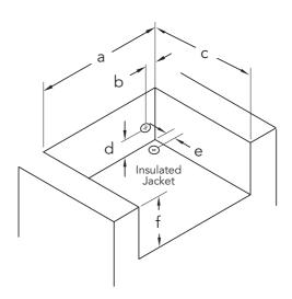
**Note:** Insulated jacket required for all grills installed into a cumbustable enclosure.
